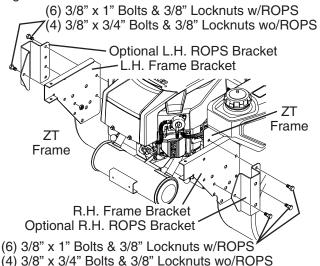
**C.** Re-install the ROPS into the ROPS mounting brackets and bolt to the frame using the four 1/2" x 3-1/4" bolts and 1/2" locknuts originally used to mount to the rear bumper. Tighten all mounting fasteners. See (Figure 9).
